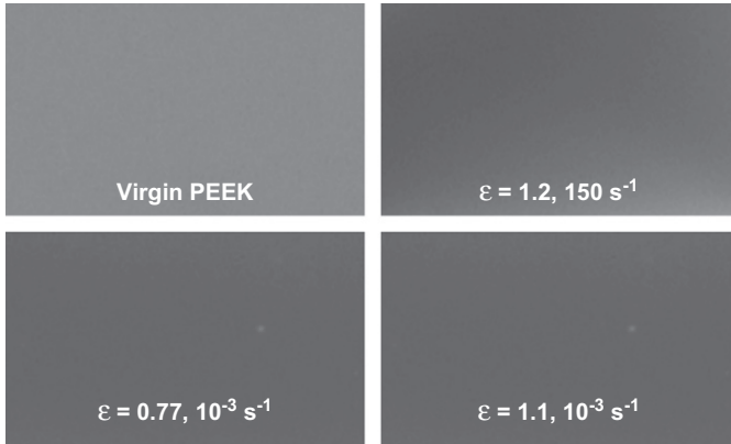
Fig. 13. Polished sections of four PEEK samples photographed under identical conditions to show the colour change associated with large-strain deformation. The grayscale value, in the range 0–255 where 255 is black, is 139 for virgin PEEK, 178 for \epsilon = 1.2 , 181 for \epsilon = 0.77 , and 181 for \epsilon = 1.1 .
